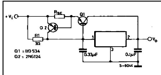
The circuit of figure 6 can be modified to provide supply protection against short circuit by adding a short-circuit sense resistor,  $R_{sc}$ , and an additional PNP transistor. The current sensing PNP must be able to handle the short-circuit current of the three-terminal regulator. Therefore, a four-ampere plastic power transistor is specified.
