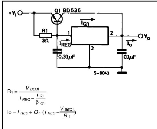
**Figure 5 :** Adjustable Output Regulator.
