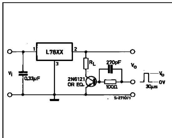
Figure 3 : Ripple Rejection.
