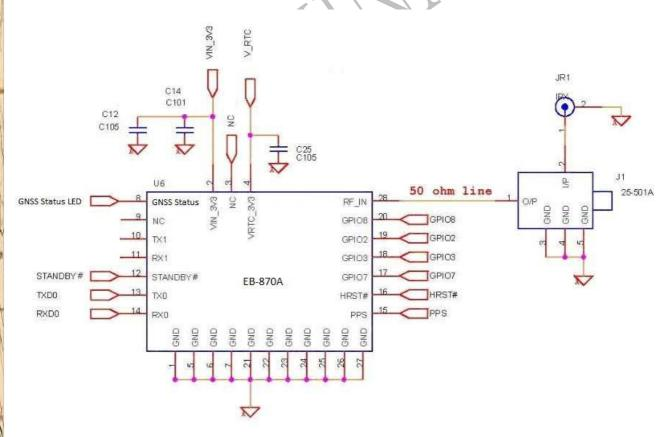
[Note 1]: VRTC\_3V3 (pin#4) could connect to 3.3V DC power supply or battery directly. (EB-870A)
