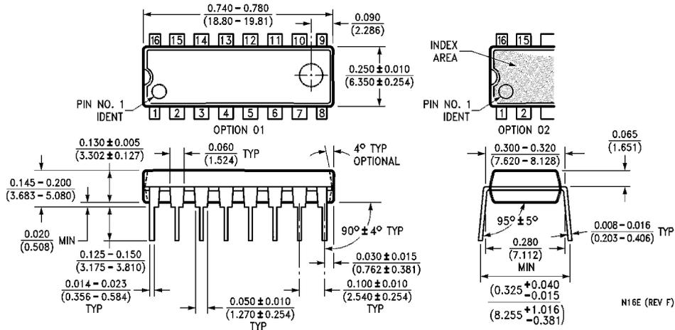
**16-Lead Molded Dual-In-Line Package (N)
