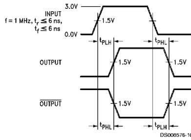
FIGURE 8. Load Propagation Delays for "LS-Type" Load
