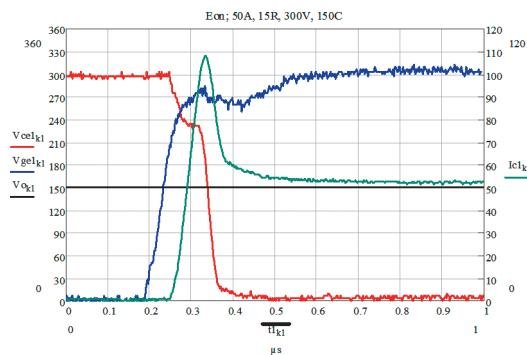
Figure 4: Trench IGBT turn-on characteristic
