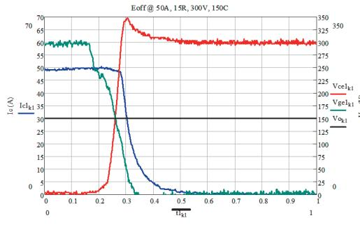
Figure 3: Trench XPT turn-off characteristic
