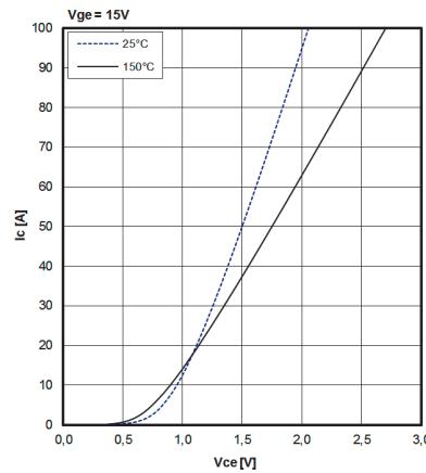
Figure 2: Trench XPT output characteristic
