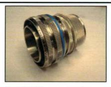
These Stainless steel firewall connectors to Rolls-Royce specification ESC15, are a development of the ESC10 connector having a rear shell designed to accept banded coupling for screens and/or heatshrink boot. Receptacles are available fitted with clinch nuts to allow easier mounting. Parts are only supplied without contacts and plugs are available with or without EMI grounding fingers. Contact used are to specification ESC30. 10-06 layout is included in ESC15 specification.
