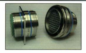
Stainless steel firewall connectors to European specification BS-EN2997. Derivative of Mil-DTL-83723 series 3 with 360° accessory teeth. Available with or without EMI grounding fingers and with or without contacts. Contact specification is EN3155.
