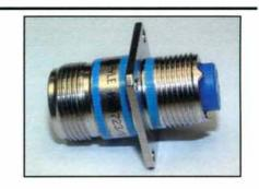
Stainless steel firewall rear-release connectors approved to MIL-DTL-83723 specification. Firewall class use only threaded coupling. Full coupling is indicated by coupling nut covering red indicator band. Plug is available with EMI grounding fingers . Versions are available with 3 or 360° accessory teeth.
