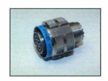
Stainless steel firewall rear-release connectors approved to MIL-DTL-38999 specification. Connection is by tri-start buttress thread with only 360° rotation to fully coupled position. Full coupling is indicated by coupling nut covering red indicator band Plug is only available with EMI grounding fingers . All parts have 360° accessory teeth.
