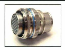
These stainless steel scoop-proof firewall connectors to Rolls-Royce ESC16 specification, are a development of the ESC11 types having a rear shell designed to accept banded coupling for screens and/or heatshrink boot. Specification dictates that parts are only supplied without contacts. Plugs are available with or without EMI grounding fingers and receptacles may be ordered with clinch nuts. Contact specification ESC30
